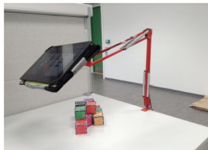
Figure 2: CogARC interaction settings: 10 cubes and a tablet PC on the base stand.
