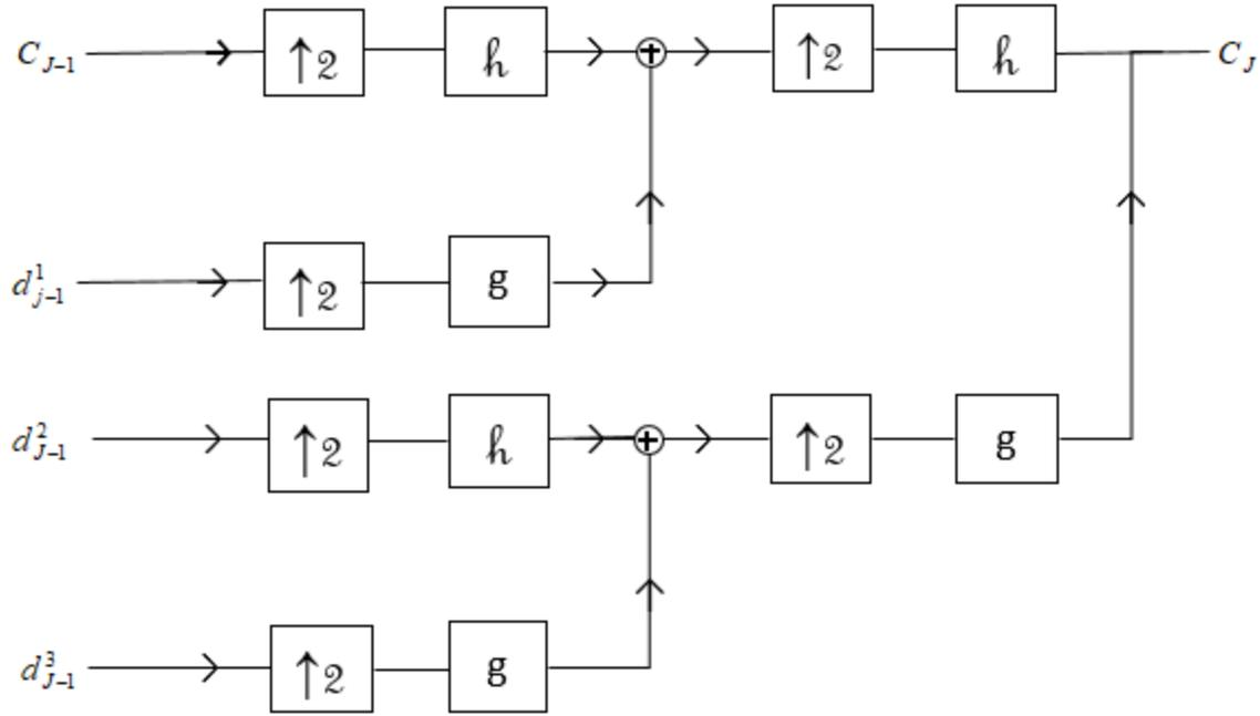
**Figure 4:** Reconstruction of  $c_J$  by inserting the zeros between the rows and columns of  $c_{J-1}$  and  $d_{J-1}^k$ , and filtering the result.
