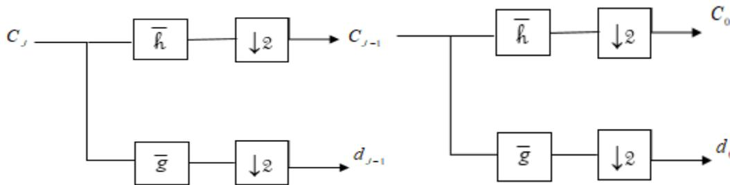
Figure 1: Analysis: filter bench
