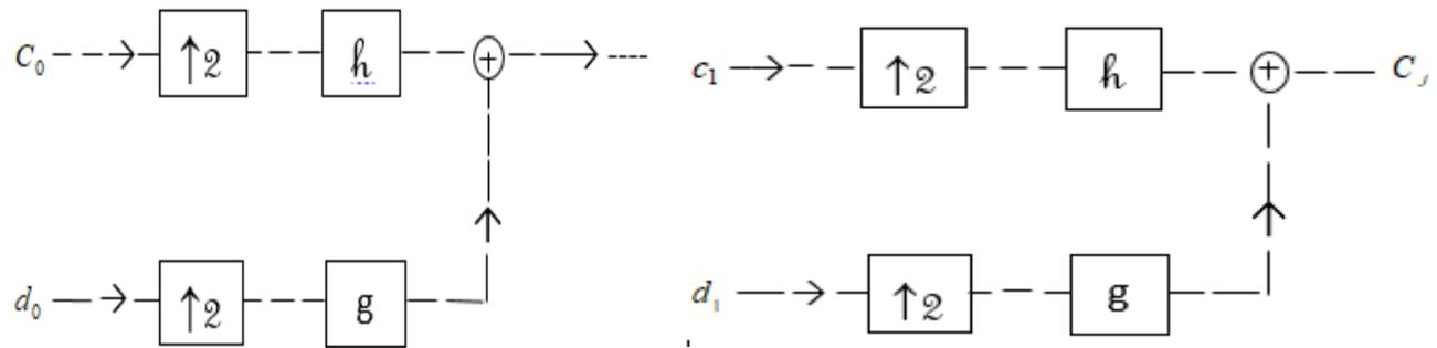
**Figure 2:** Synthesis: filter bench
