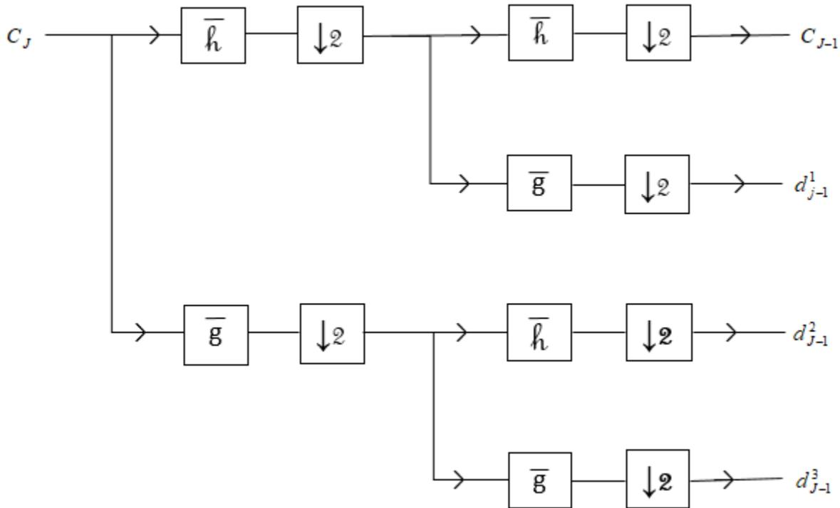
**Figure 3:** Decomposition of  $c_j$  into 6 convolution groups and one-dimensional sub-samples along the rows and columns of the blurred image.
