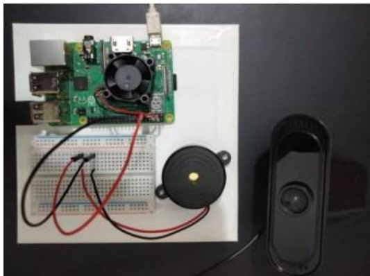
Fig. 8. The example of piezo buzzer set up for the FACID system
