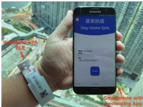
Fig. 2. An example of home quarantine monitoring system StayHomeSafe deployed in Hong Kong
