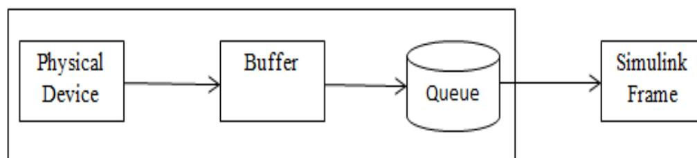
Figure 1: The From Audio Device Block
