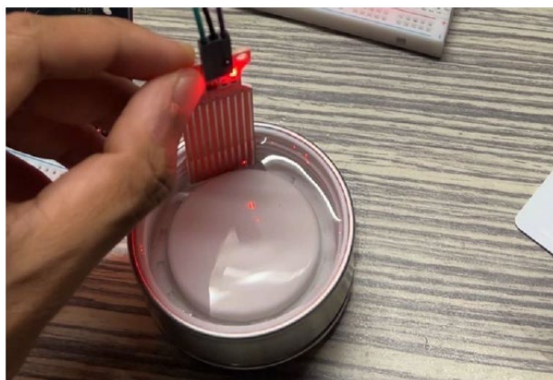
Fig. 11. The water detection as a flood system alert
