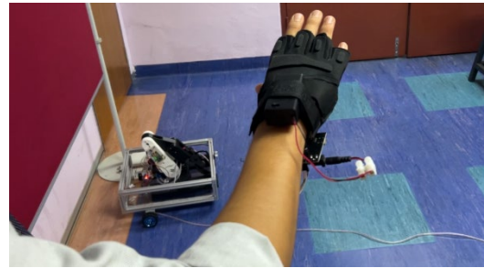
(j) Automatically stopped to avoid the wall
